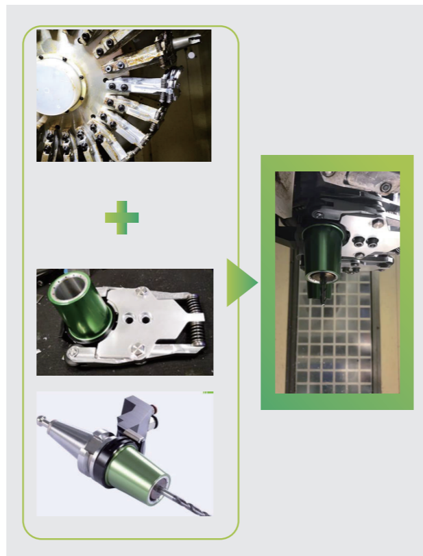
Tool Change System of Ring-Type Nozzle
